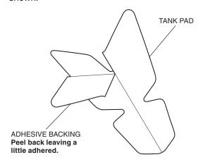
5. Attach the tank pad as shown.
