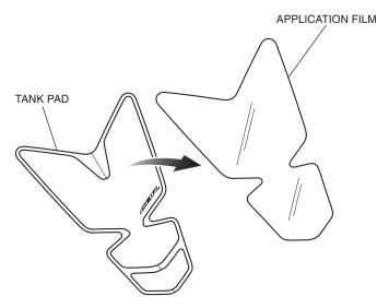
3. Arrange the tank pad as shown and mark with masking tape.
