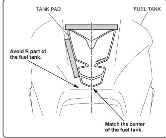
4. Peel off the adhesive backing on the tank pad as shown.
